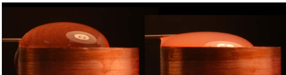
Fig. 13. Photographs of advancing droplets: water on copper (left) and 1.02 g/L alumina/water nanofluid on nanoparticle fouled copper (right).
